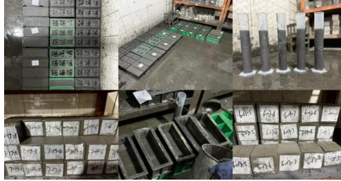
Figure 2 Indoor confirmation test block bleeding
